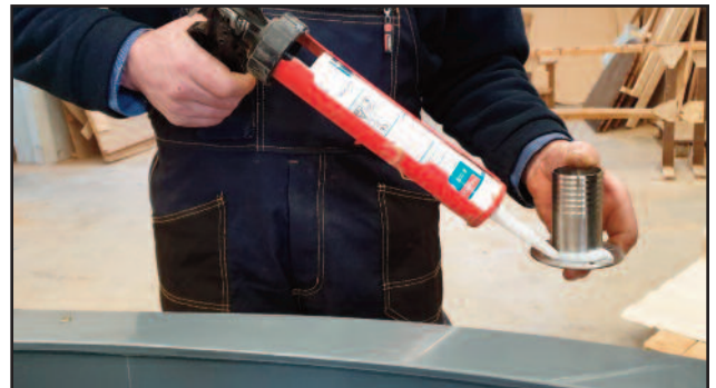
11. Silicone pipe spigots around the middle and place and position in side holes from the inside:
